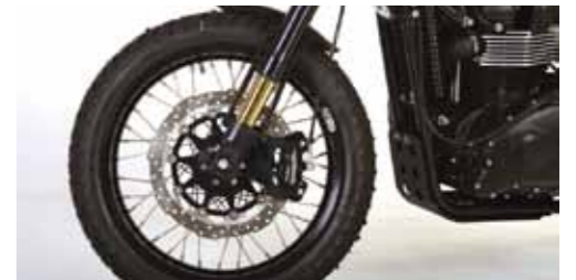
Ohlins Upside down forks with Sun aluminium racing rims with a single 4-piston Beringer racing brake calliper.
